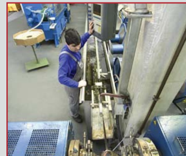
Thermoplastic co- or mono-extrusion with or without steel or wire carrier
