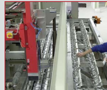
Linear laser cutting robot with double laser unit
