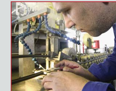
Splicing of an edge protector with a sponge rubber sealing
